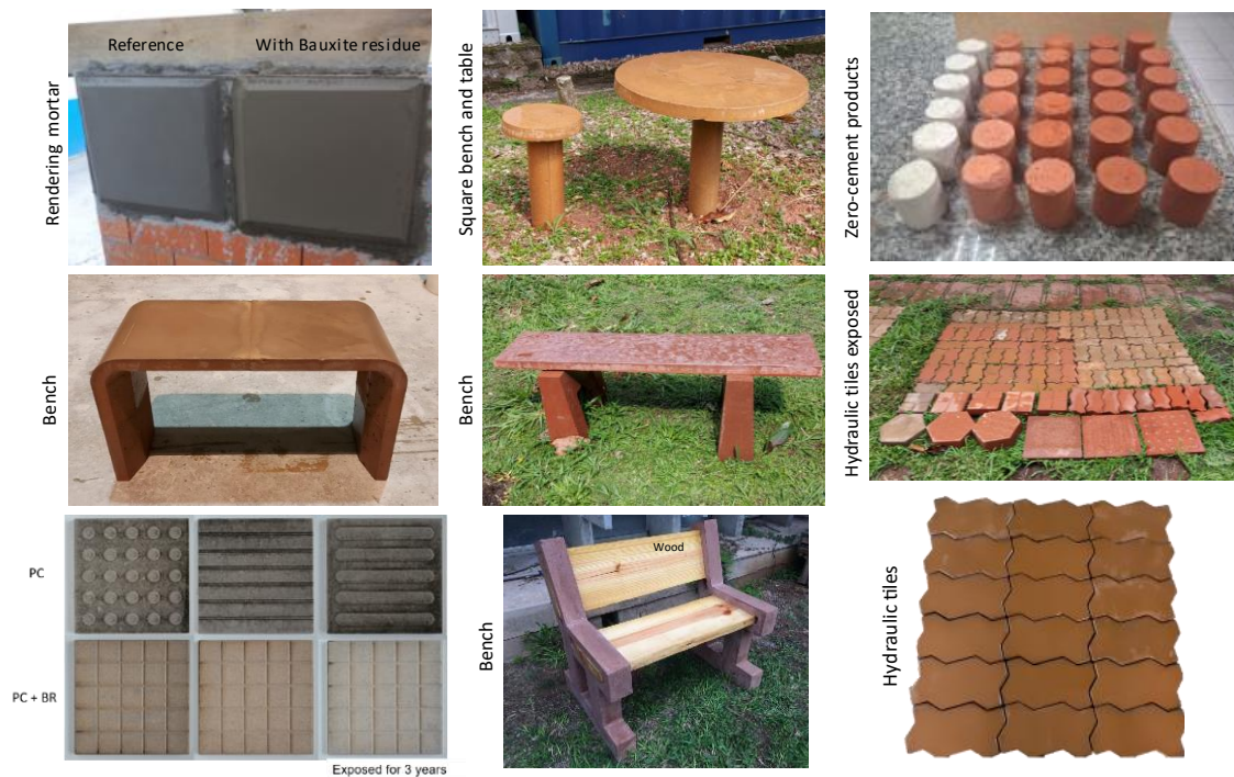
Figure 4. Components developed for monitoring after exposure to environmental conditions.
